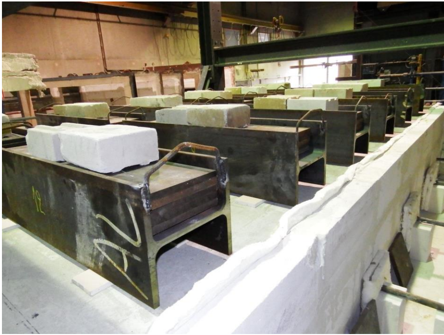
Fig. 1. Steel beams rotated by 90° and dead weights inside (photo by: F. Dumont, Uni. Liège)
