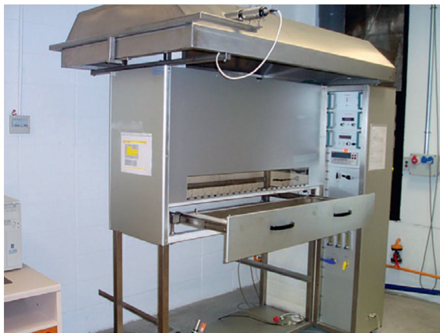
Figure 1: Test apparatus according to EN ISO 9239-1. The photo is taken by one of the participants.
