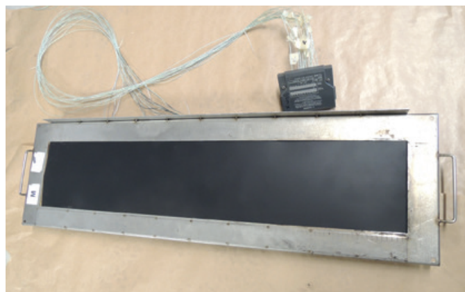
Figure 2: Calibration board used in the round robin exercise. The front side is shown in the left photo, and the rear side with the mounted thermoelements is shown in the right photo. Photos: SP Fire Research, Borås.
