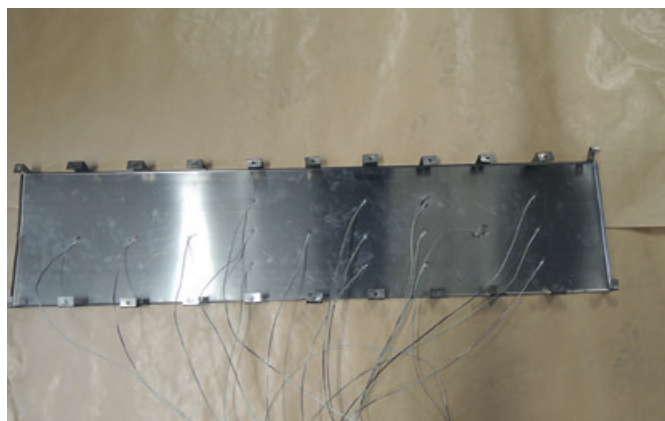
Figure 2: Calibration board used in the round robin exercise. The front side is shown in the left photo, and the rear side with the mounted thermoelements is shown in the right photo. Photos: SP Fire Research, Borås.
