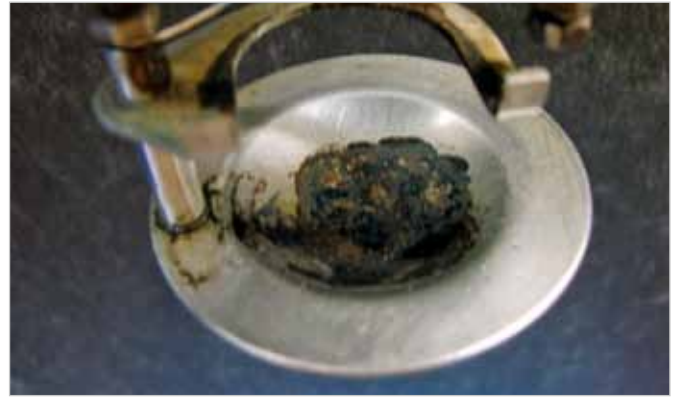
Material 1 (copolyamide) after the test.
