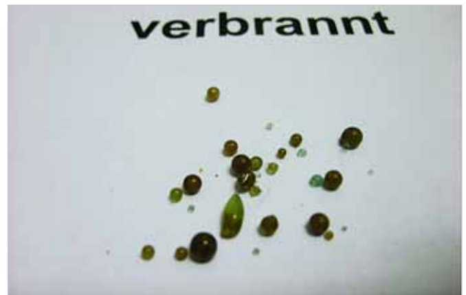
Material 2 (mineral wool) after the test.
