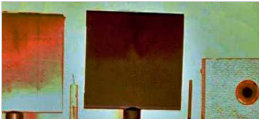
Figure 3. Two TCs and a Gardon gauge heat flux meter mounted in front of a radiant panel. The measured temperatures are shown in Figure 4.
