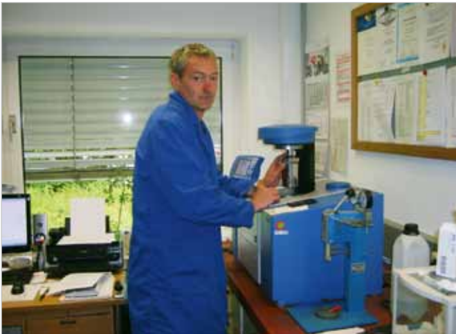
Calorimetric bomb being placed before the test.
