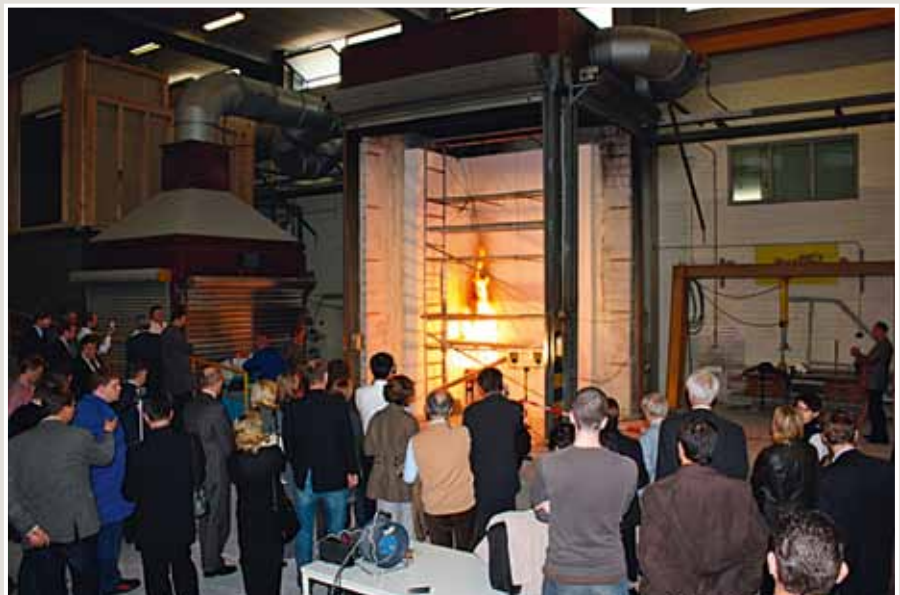
Large scale façade test for determining the reaction to fire behaviour of external thermal insulation composite systems with rendering (ETIC).
