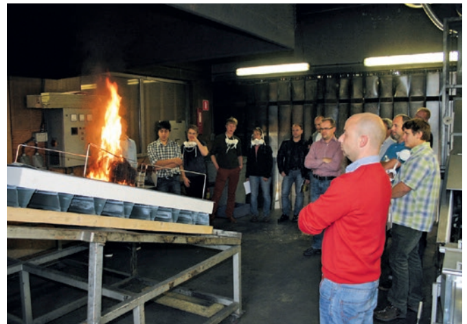
Testing according to CEN/TS 1187 test method 1. The left photo shows the burning wood wool basket placed on a test specimen of roofing on a substrate of thermal insulation material. The right photo shows testing according to the method during an EGOLF harmonisation course at Kiwa BDA Testing B.V in 2013. Photos: Kiwa BDA Testing B.V.
