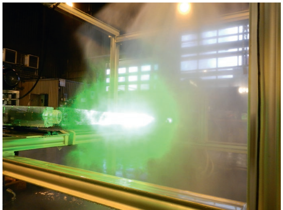
PIV, a laser measurement technology for determining detailed information of particles in a flow field.
