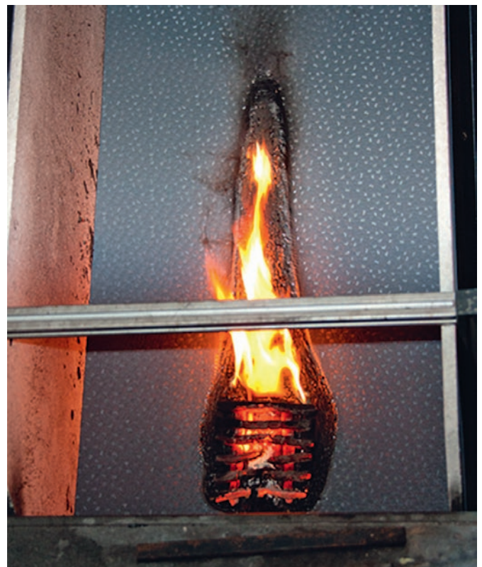
Testing according to CEN/TS 1187 test method 2. The left photo shows the test apparatus and the burning wood crib being placed on a test specimen. The right photo shows the burning crib on the specimen during test. Photos: Thor Kr. Adolfsen, Norwegian Fire Protection Association.
