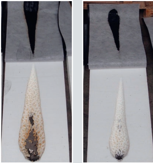
Test method 2, Sample 3: Bitumen roofing on EPS insulation. The photos show typical damaged specimens, the roofing is folded backwards and we see the underside of the roofing in the upper part of the photos. Specimen tested at wind speed 2 m/s to the left, and at 4 m/s to the right.
