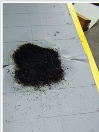
Test method 1, Sample 1: PVC roofing on EPS insulation with glass fleece between the layers. The photos show typical damaged specimens. Damaged roof water proofing material to the left, damaged EPS insulation to the right.
