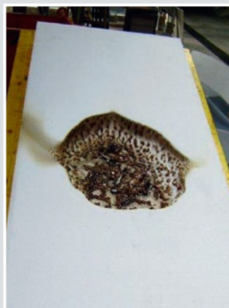
Test method 1, Sample 1: PVC roofing on EPS insulation with glass fleece between the layers. The photos show typical damaged specimens. Damaged roof water proofing material to the left, damaged EPS insulation to the right.
