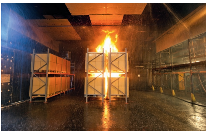
Test of sprinkler system for a warehouse.
