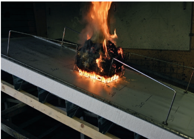
Testing according to CEN/TS 1187 test method 1. The left photo shows the burning wood wool basket placed on a test specimen of roofing on a substrate of thermal insulation material. The right photo shows testing according to the method during an EGOLF harmonisation course at Kiwa BDA Testing B.V in 2013. Photos: Kiwa BDA Testing B.V.
