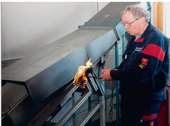
Testing according to CEN/TS 1187 test method 2. The left photo shows the test apparatus and the burning wood crib being placed on a test specimen. The right photo shows the burning crib on the specimen during test. Photos: Thor Kr. Adolfsen, Norwegian Fire Protection Association.
