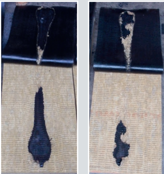
Test method 2, Sample 4: Bitumen roofing on mineral wool insulation. The photos show typical damaged specimens, the roofing is folded backwards and we see the underside of the roofing in the upper part of the photos. Specimen tested at wind speed 2 m/s to the left, and at 4 m/s to the right.
