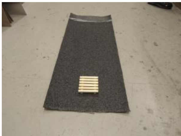
Photo 2: Position of crib during test.
